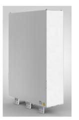
Power Module 2: Voltage category: 380 / 500 / 690 V Switching: DC/AC Power: 1,000 - 2,000 kW Liquid-cooled Cooling: Temperature range: -40 to 50 °C IP rating: IP21 Weight: 104 kg Dimensions (H/W/D): 890 / 215 / 580 mm Also available in: AFE
